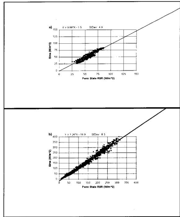
**Figure 2.** Comparison of RSR and SIROS 5-min. averages of diffuse SR for a) clear and b) all-sky measurements. Standard deviations are calculated from linear fit shown.
