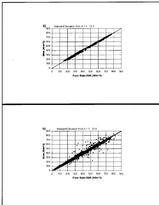
**Figure 1.** Comparison of RSR and SIROS 5-min. averages of total SW for a) clear and b) all-sky measurements.
