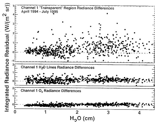
**Figure 3.** Integrated radiance residuals between the measured AERI-00 radiance and the LBLRTM calculated radiance as a function of radiosonde column water vapor for the transparent regions (top), H<sub>2</sub>O lines (middle), and O<sub>3</sub> lines (bottom).
