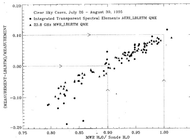
**Figure 4.** Fractional error for both the longwave transparent region radiances and the 23.8 GHz brightness temperatures as a function of the ratio of the MWR water vapor product to the BBSS measured water vapor column for the time period July 26 - August 30, 1995.
