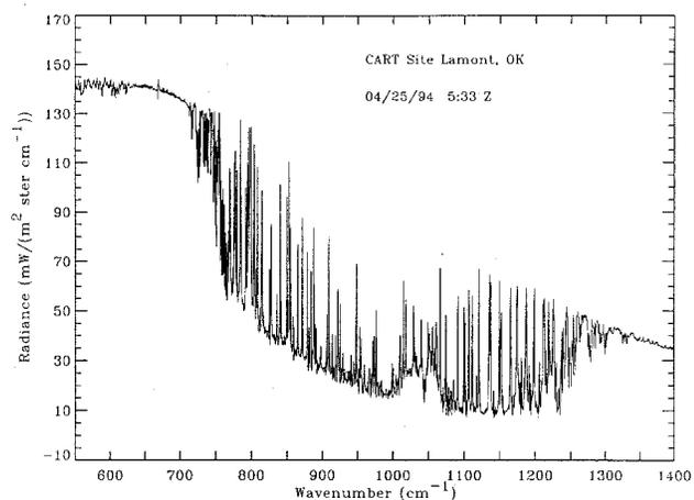
**Figure 1.** AERI-00 downwelling radiance spectrum measured April 25, 1994.
