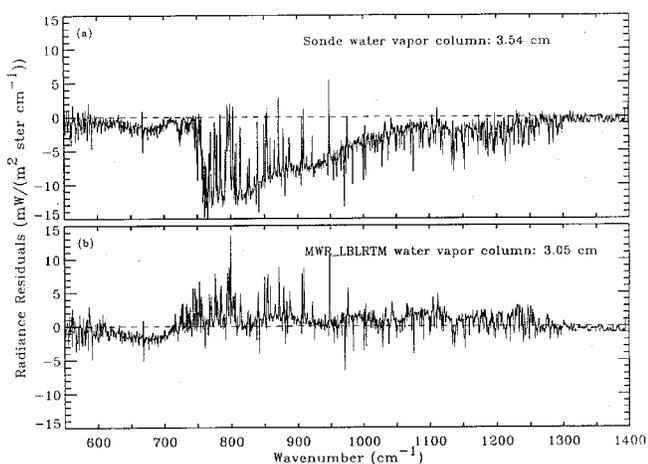
**Figure 6.** AERI-01 - LBLRTM residuals for 08:30Z July 28, 1995 using (a) sonde measured water vapor and (b) LBLRTM retrieved water vapor column as model input.
