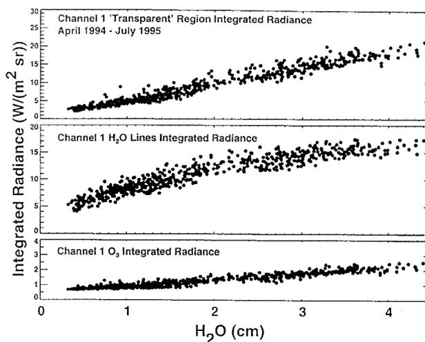
**Figure 2.** AERI-00 integrated measured radiance as a function of radiosonde column water vapor for the transparent regions (top), H<sub>2</sub>O lines (middle), and O<sub>3</sub> lines (bottom).
