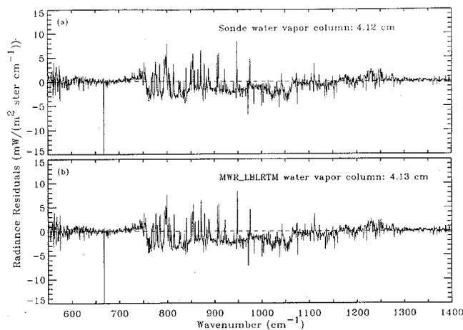
**Figure 5.** AERI-01 - LBLRTM residuals for 11:29Z August 17, 1995 using (a) sonde measured water vapor and (b) LBLRTM retrieved water vapor column as model input.
