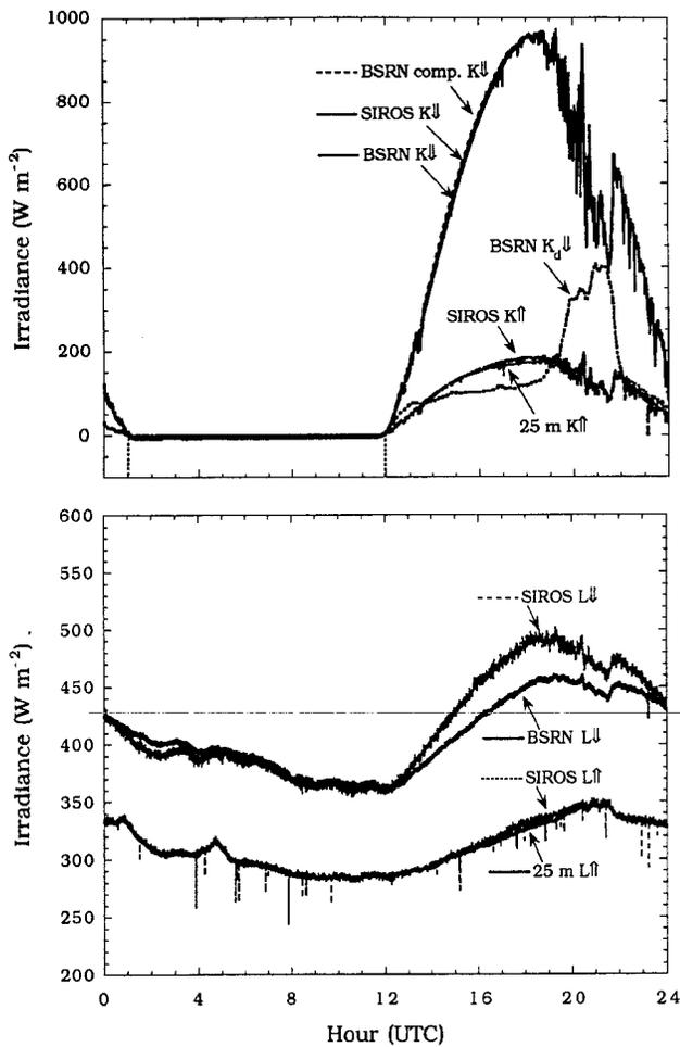
**Figure 3.** Irradiance observations made with pyranometers, pyrgeometers, and a pyrheliometer during April 18, 1994, where “K” indicates solar radiation, “L” longwave radiation, the downward pointing arrow to downwelling radiation, the upward pointing arrow to upwelling radiation, “comp.” to the component sum of diffuse plus direct-beam irradiance on a horizontal surface, and the subscript “d” to diffuse solar radiation seen with a shaded pyranometer.
