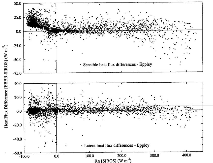
**Figure 2.** Differences between 30-min-average surface flux estimates from the EBBR and recalculated fluxes using the SIROS net radiation values (with the Eppley factory calibration coefficients) for (a) sensible heat flux and (b) latent heat flux for December 1994, January 1995, and February 1995.
