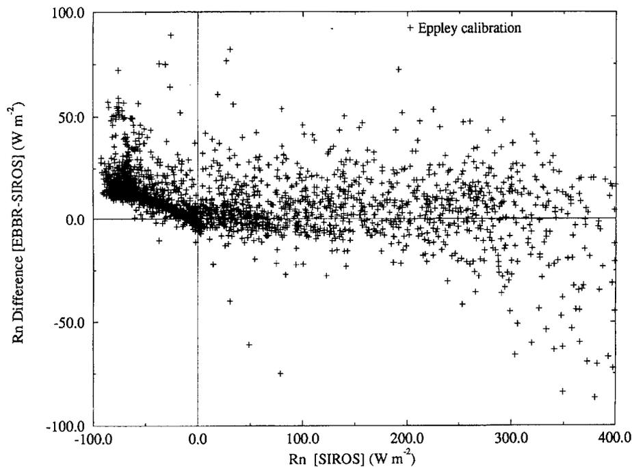
**Figure 1.** Differences between 30-min-average net radiation estimates from the central facility EBBR and SIROS during December 1994, January 1995, and February 1995 versus the SIROS net radiation values. The SIROS net radiation estimates were computed with the Eppley factory calibration coefficients.
