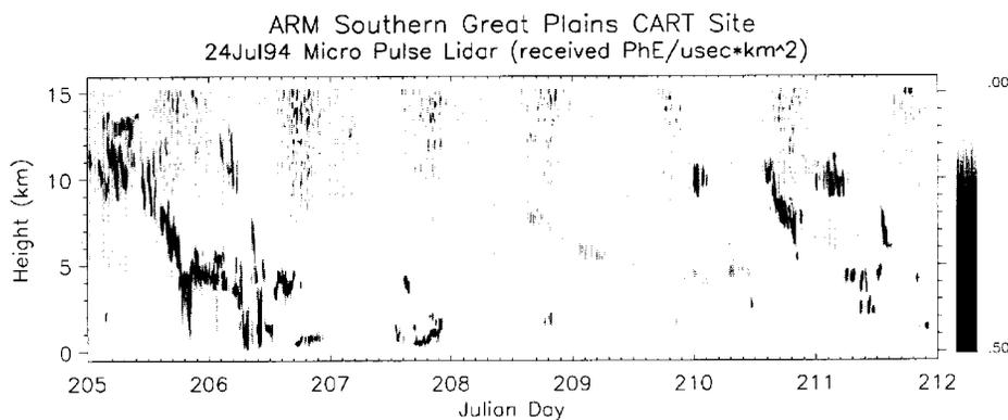
**Figure 1.** Image of MPL data from the Oklahoma CART site. The data is displayed in range corrected format but with no near range overlap correction of the near ground signal. Similar browse images for all MPL data are to be made available in GIF format.
