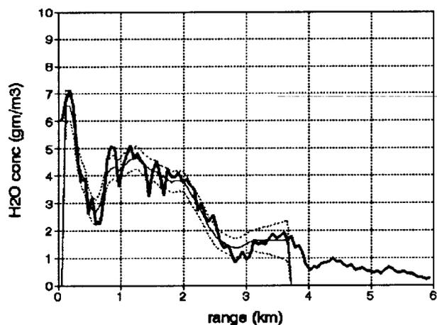
**Figure 1.** Performance of a “small” CO<sub>2</sub> heterodyne system with a 0.3-m mirror pointing vertically and focused at 3 km, integrating the return from 5-mJ, 1-kHz lidar over 10 secs (50 J total). The heavy solid line shows the “true” water vapor concentration, the solid line shows the lidar estimate, and the dotted lines are  $\pm 1 \sigma$  around the estimate. Only 60 (out of 100) range gate data points are processed.
