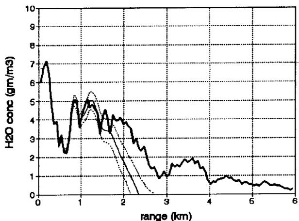
**Figure 2.** Performance of 50-J CO<sub>2</sub> direct detection lidar for comparison with data of Figure 1. Using a TEA laser, this system might be realized with a 0.5-J laser operating at 100 Hz for 10 secs. A 1-m diameter receiving dish is assumed.
