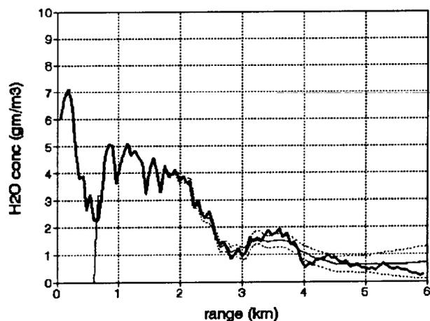
**Figure 4.** Performance of 300-J (e.g., 100 mJ at 10 Hz for 5 mins) direct detection 2- $\mu$ m lidar for comparison with data of Figure 3. A 1-m receiver is assumed. The noise equivalent power (NEP) of the photodetector does not take account of daylight background.
