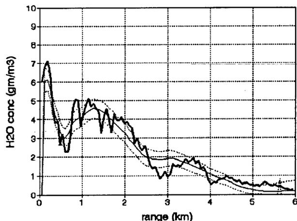
**Figure 3.** Performance of a 300-J 2- $\mu$ m heterodyne lidar (5 mJ at 200 Hz for 5 mins) pointing vertically and focused at 5 km. Transmitter and receiver dishes are assumed to be of diameter 0.5 m. Improved results at shorter ranges could be obtained by focusing.
