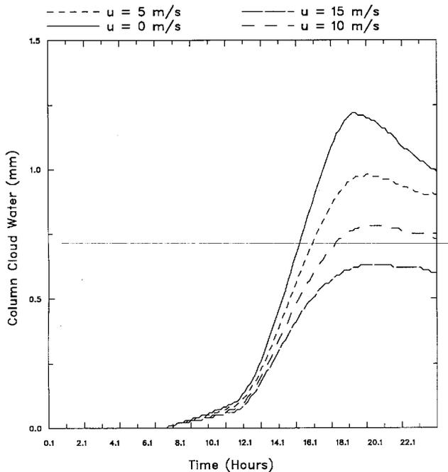
**Figure 1.** Simulations of column cloud water by the single column model with different horizontal wind speeds. The model was initialized with relative humidity that decreases from 90% to 60% from the surface to 6 km, and is driven by a fixed vertical velocity of  $1 \text{ cm s}^{-1}$ .
