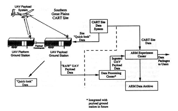
Figure 1. Functional elements of the ARM/UAV system.
