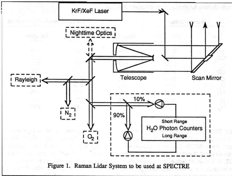
Figure 1. Raman Lidar System to be used at SPECTRE
