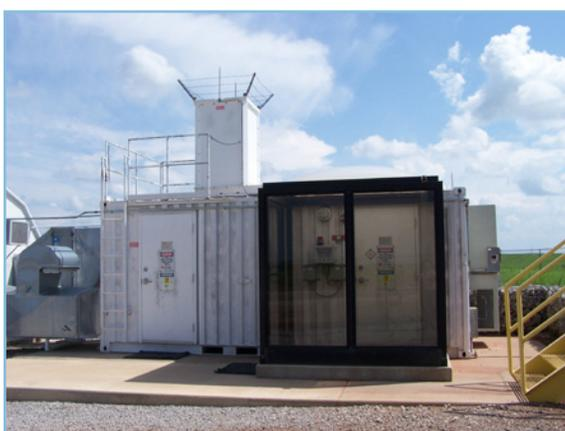
Developed for ARM as the first turn-key operational Raman lidar in the world, the original ARM Raman lidar has operated nearly autonomously at the SGP site since 1996. Recovery Act upgrades include a new laser system, a new beam-expanding telescope for the transmitted beam, and updating the computer operating system and the lidar control software.
