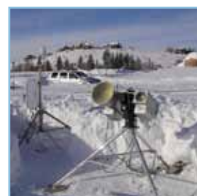
The high-volume precipitation spectrometer (front) measures the number and size of precipitation particles, including snowflakes, from 150 microns to 1.92 centimeters in size. This is the only aircraft research instrument of its kind that provides complete digital images of precipitation particles up to nearly 2 centimeters in size.
