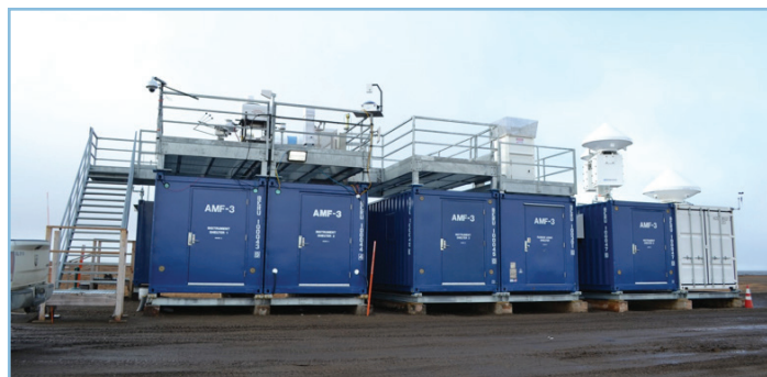
The AMF3 instrument collection onsite includes a downwelling radiometer, total sky imager, Raman lidar, W-band ARM cloud radar, and the Ka- and W-band scanning ARM cloud radars, all instrumental in collecting data on clouds, aerosols, and the sun's rays.
