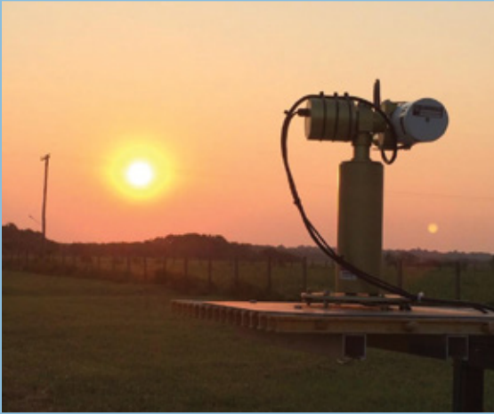
Partially obscured by aerosols in the atmosphere due to a forest fire northeast of Manaus, the sun sets over the ARM Facility's Mobile Aerosol Observing System located southwest of Manaus, Brazil. At the T-3 site in Manacapuru, a sunphotometer measures the optical density of the aerosols in the column.
