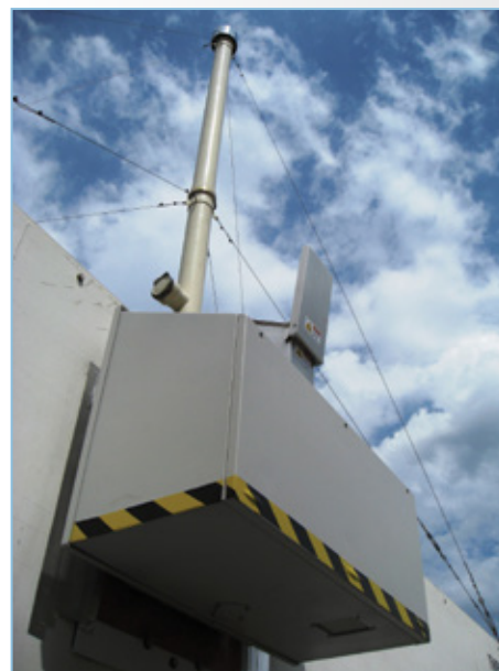
ARM Mobile Facility instrumentation was installed in June 2011 at the Aryabhata Research Institute of Observational Sciences (ARIES) Observatory in Nainital, India, for the Ganges Valley Aerosol Experiment (GVAX). Shown in this photo are the stack for the aerosol observing system (AOS, top) and the optics enclosure for the atmospheric emitted radiance interferometer, or AERI.
