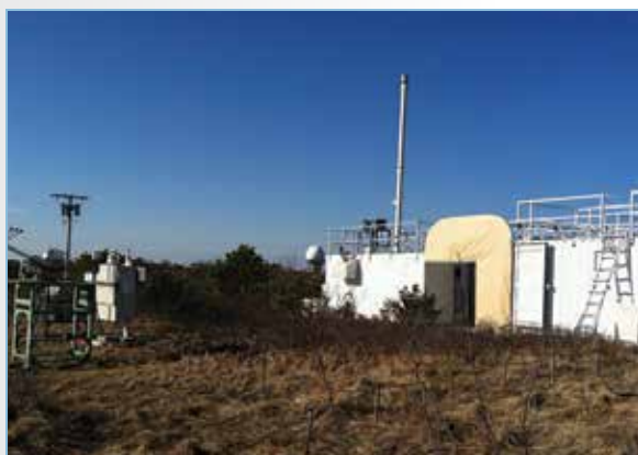
The AMF1 was deployed on Cape Cod National Seashore during TCAP. This view, facing west, shows several radiometers operating on the left, and the Mobile Aerosol Observing System on the right.
