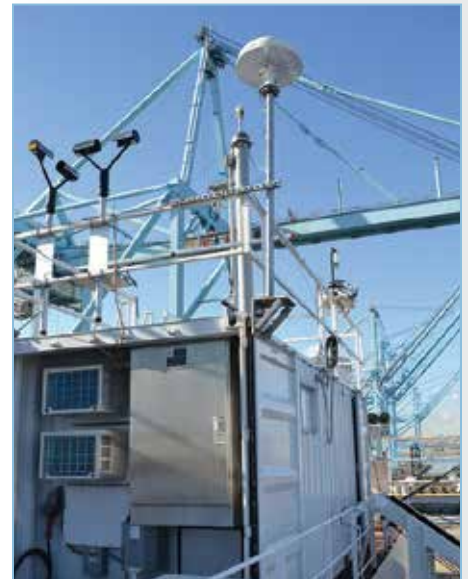
The aerosol observing system is the primary ARM platform for in situ aerosol measurements at the surface and was used aboard the ship Horizon Spirit during the MAGIC campaign.
