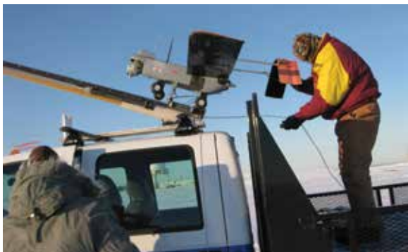
Because of its small size and light weight (72-inch wingspan and weighing about 22 pounds), the Bat-3 is launched using a bungee-powered catapult from the roof of a vehicle and can land autonomously on fixed wheels. Its modular design fits into two suitcase-sized containers.
