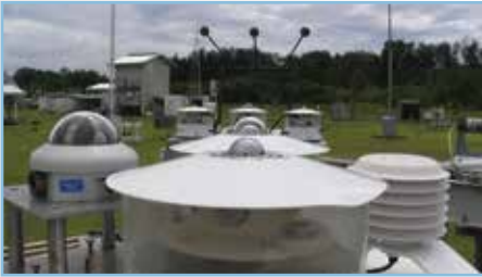
Radiometers at ARM's TWP Manus site gathered data in support of AMIE-Manus.
