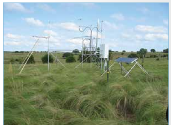
EBBR systems like the one shown here produce 30-minute estimates of the vertical fluxes of sensible and latent heat at the local surface.
