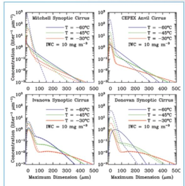
The retrieved mean effective  $\beta$  was found to be 1.065 for thin cirrus having temperatures  $< -35$  Celsius. Based on this value, PSD were retrieved (solid) and compared with corresponding PSD given by the original PSD scheme (dashed). The retrieved PSD have lower concentrations of small ice crystals, with bimodality increasing with increasing temperature.
