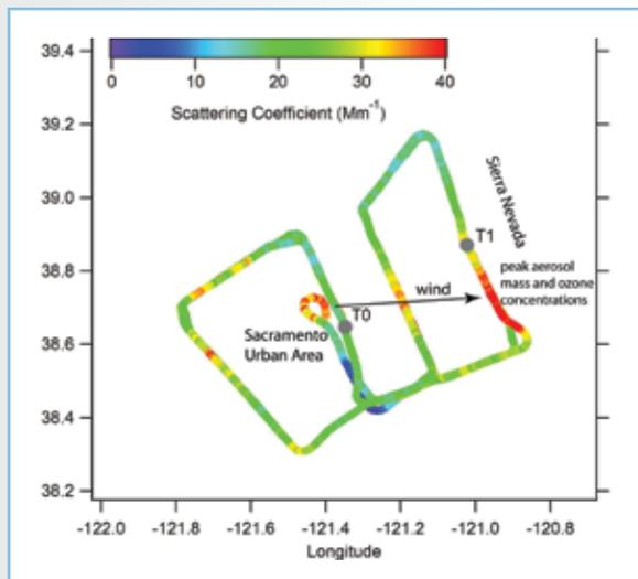
Spatial distribution of aerosol light-scattering coefficient for the 500 nanometers (green) wavelength on the afternoon of June 28, 2010, showing the presence of the Sacramento aerosol plume in the Sierra Nevada foothills area to east of the urban source region. The measurements were taken aboard the G-1 aircraft. The locations of the two ground sites, T0 and T1, are also featured.
