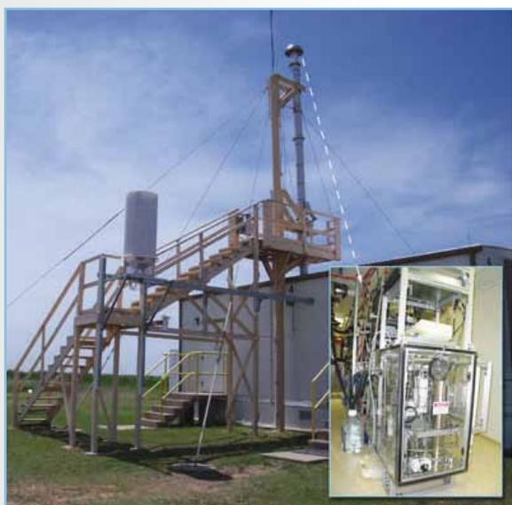
Over 4 years of data from the tandem differential mobility analyzer (TDMA), including an external value-added product, became available online at the ARM Data Archive in FY 2010. Data from the TDMA, located at the ARM Facility's SGP site, measure aerosol dry-size distribution and size-resolved hygroscopic growth rate factors (i.e., relative growth of dry aerosol particles of a given size when exposed to a relative humidity of 85%).
