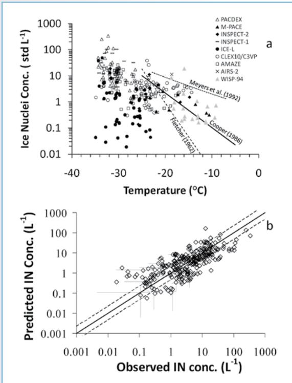
(a) IN number concentration for mixed-phase cloud conditions versus temperature from nine studies. Data points are 5–30-minute averaged data. Single variable (T, RH) parameterizations are labeled and plotted over the data. (b) Relation between observed IN from panel (a) to IN predicted by the new parameterization linking temperature and aerosol concentrations larger than 0.5 microns. Dashed lines indicate observations (62%) within a factor of 2 of 1:1 line.
