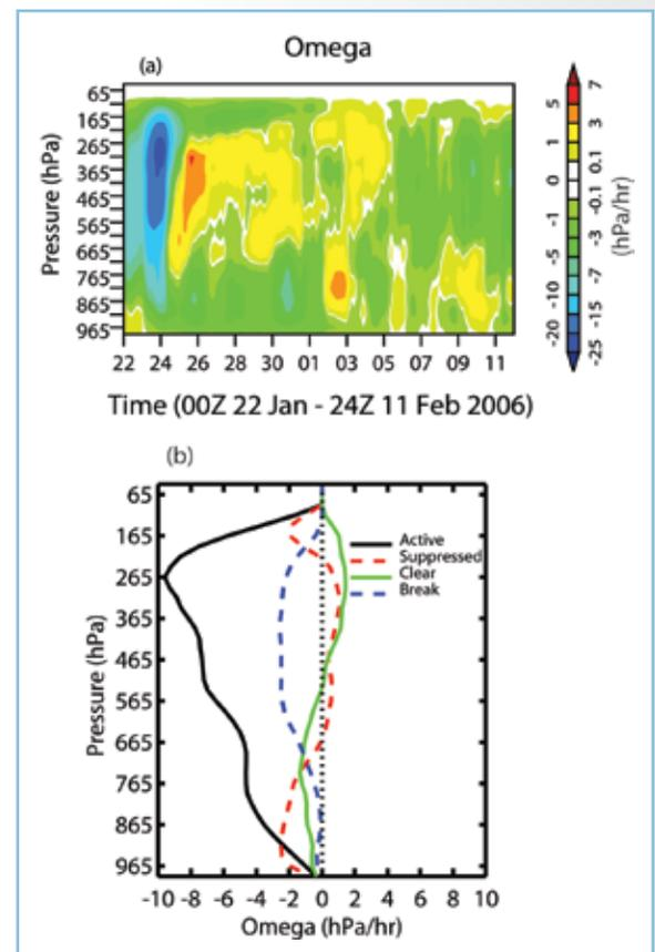
Analyzed vertical velocity ( $\omega$ ): (a) temporal evolution; (b) averaged profiles for different periods. Significant variations between the four distinct synoptic regimes are shown in the vertical velocity profiles observed during TWP-ICE.
