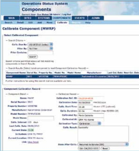
The Common Calibration Database provides a quick way to view calibration information associated with an instrument and its subcomponents.
