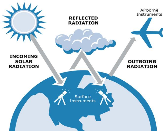
Researchers use data collected from ARM ground-based and airborne instruments to study the natural phenomena that occur in clouds and aerosols and how those conditions affect incoming and outgoing radiative energy.
