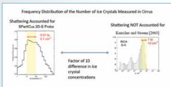
The data plot on the left shows the frequency distributions of ice crystal concentrations measured during SPARTICUS compared to similar statistics in earlier campaigns, shown on the right.
