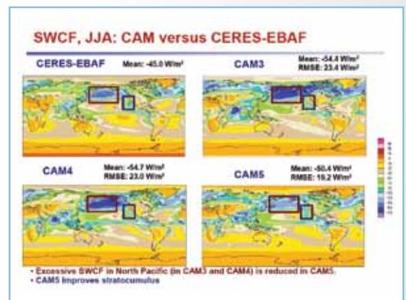
Shortwave cloud forcing for three versions of the NCAR Community Atmosphere Model (CAM) with CERES observations at upper left for June–August 2010. The latest model, CAM5 (at lower right), shows improvement in both mean error and root mean square error (RMSE), with notable improvement in the tropics, the North Pacific, and the stratocumulus region over the Eastern Pacific. Figure courtesy of NCAR.
