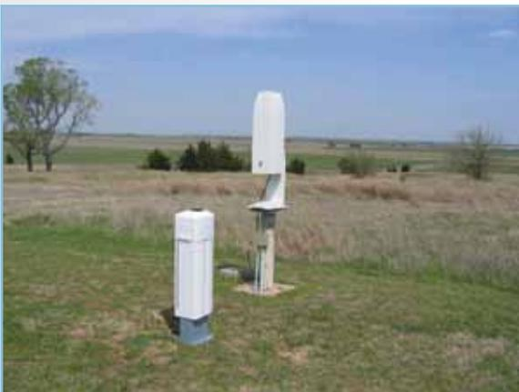
After a 3-day period of side-by-side operations and acceptance testing, the new CL31 ceilometer (foreground) officially replaced the older CT25K model on April 16, 2010, at the SGP site.
