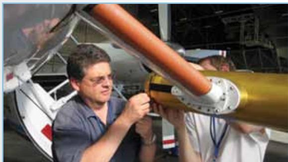
AAF Technical Director Beat Schmid, left, and Operations Lead Jason Tomlinson, right behind the probe, adjust the cloud aerosol and precipitation spectrometer on the G-1.
