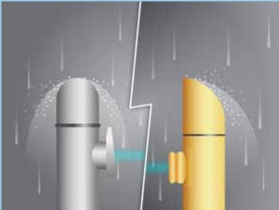
Newer aircraft probes were designed to potentially minimize the shattering effect that previously resulted in a disproportionate amount of smaller particles being measured by the sensor beam.
