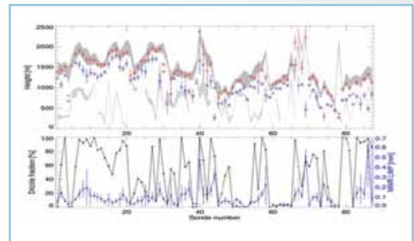
The upper panel shows cloud boundaries (base from the ceilometer [blue] and top from the WACR [red]) averaged over 2 hours surrounding sounding times, superimposed on the soundings inversion and transition layers (dark and light shadings, respectively). The lower panel shows the fraction of the 2 hours that experienced drizzle (black) and the 2-hourly averaged LWP from the MWR (blue). In both panels, vertical lines represent the 2-hourly standard deviations of the measurements.
