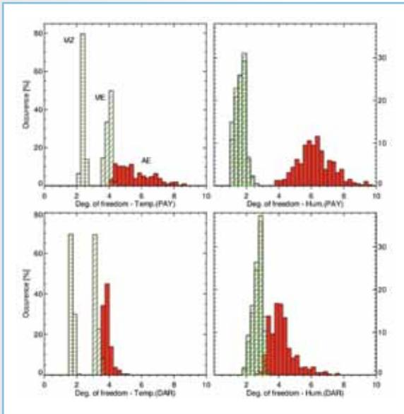
The degrees of freedom of signal in the microwave (zenith observations only [MZ] and zenith plus elevation scanning [ME]) and infrared (AE) observations from Payerne and Darwin sites, with temperature shown in the left-hand panels and humidity in the right-hand panels. The use of the elevation scans doubled the information content in the microwave retrievals. In most cases, the infrared retrievals have much larger information content than the microwave retrievals.
