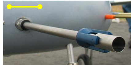
Aerosol inlet & splitter (150 g) → unbiased aerosol sampling
