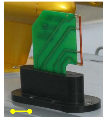
LWC probe (450 g) → Cloud water ( \text{g m}^{-3} )
