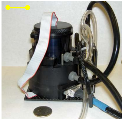
Aethalometer (820 g) → absorbing aerosol
