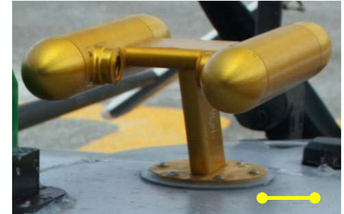
Cloud Droplet Spectrometer (1.4 kg) → distr. 1 < D < 50 \mu\text{m}
