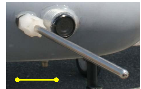
Gust probe (400 g) & video camera (280 g) → turbulence & cloud targeting
