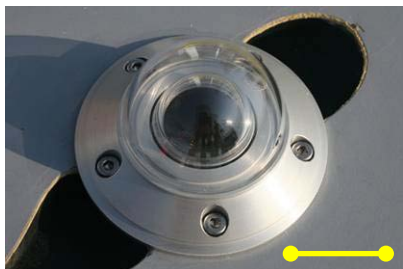
Pyranometer (190 g) → irradiance 0.3 - 2.8 \mu\text{m}
