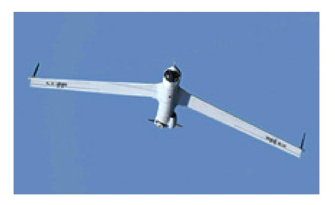
In Situ A 20 (Boeing Scan Eagle); >45,000 flight hours, mostly in Iraq; 20+ hour flight duration; wing span just over 10 feet.
