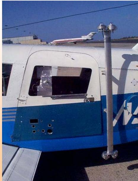
Handheld Sun Photometer Measurements From Ships and Planes
