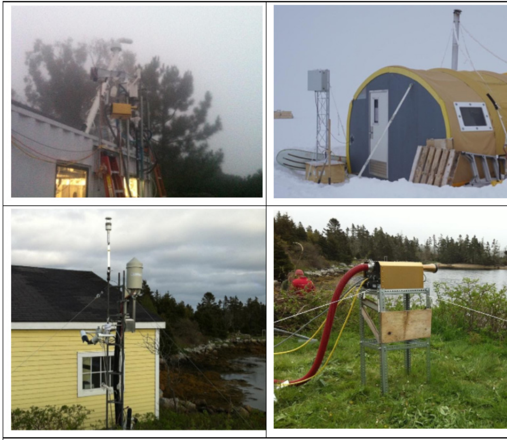
Figure 3. Russell instrumentation van deployed at Mt. Soledad in 2012 with droplet probes sampling in cloud (top left); Lubin spectroradiometer at Siple Dome Field Camp, Antarctica, in 2020 (top right); Environment Canada Brechtel CVI (bottom left) and Chang fog drop monitor (bottom right) deployed at Halifax, Canada, in 2016.
