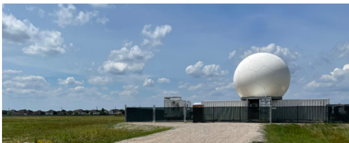
This ARM radar in Pearland, Texas, tracked convective cloud cells as part of the TRACER campaign.
