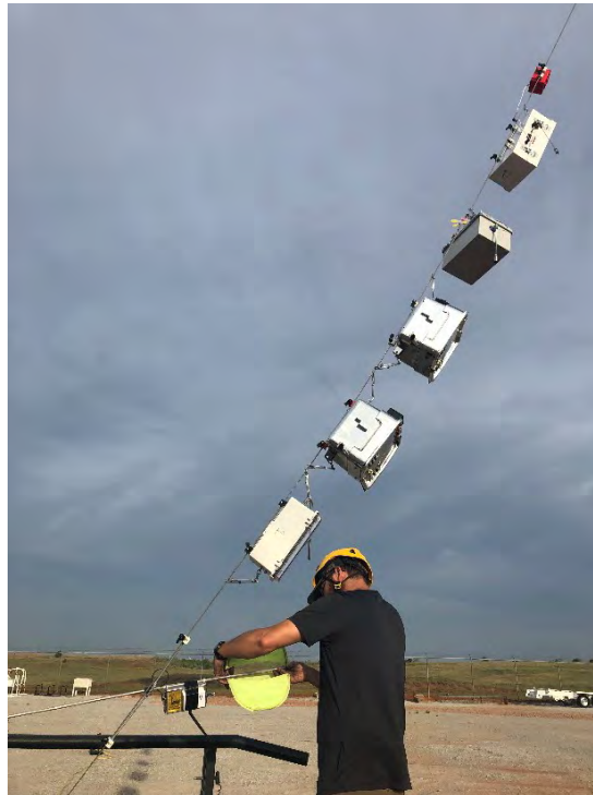
New aerosol sensors being flown on the tethered balloon system has increased ARM's ability to provide information about the vertical structure of aerosol properties through the planetary boundary layer.
