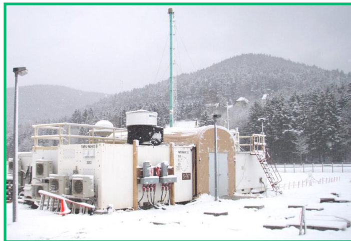
The first ARM Mobile Facility, pictured here in Germany's Black Forest, consists of instruments, operations shelters, and data and communication systems.
